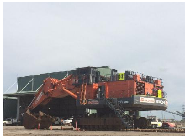
Hitachi EX5500 Excavator mobilised on site
